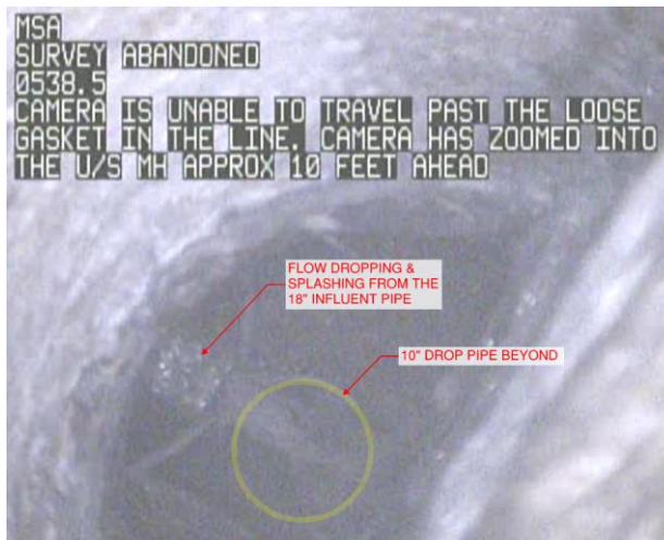
CCTV Footage Looking Upstream Into MH 13
