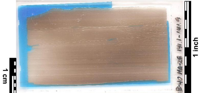
Thin section slide of medium gray shale Very thin lamination with white quartz silt-bearing layers. Blue epoxy impregnation indicates 0% intergranular porosity, but fracture porosity along parting.
