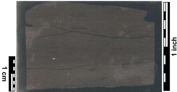
Billet of gray shale Mudstone with irregular parting along bedding highlighted by blue epoxy impregnation.
