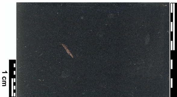
Billet of dark gray pyritic carbon-rich shale Black-when-wet shale
