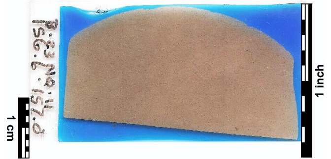
Thin section slide of massive gray siltstone Featureless isotropic and homogeneous siltstone. Blue epoxy impregnation indicates 0% porosity.
