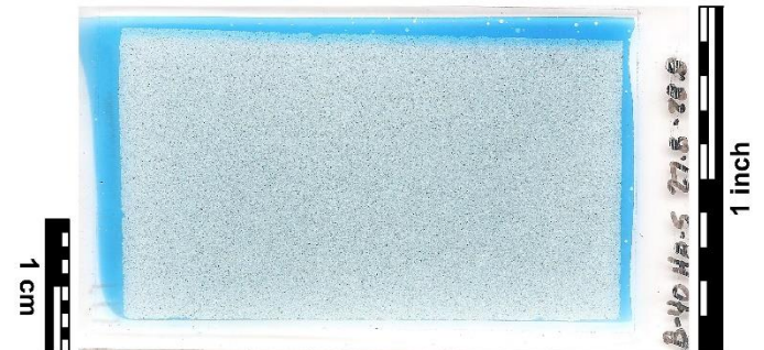
Thin section slide of fine-grained quartz arenite sandstone Note very consistent grain size (well-sorted) and blue epoxy impregnation indicating 8% intergranular porosity.
