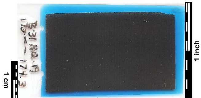
Thin section slide of dark gray shale Homogeneous dark mudstone. Blue epoxy impregnation indicates 0% observable intergranular porosity.
