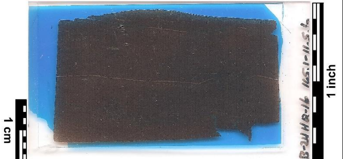
Thin section slide of dark gray weakly pyritic shale Nearly opaque with organic material. Note wavy shaley parting. Blue epoxy impregnation indicates 0% porosity.
