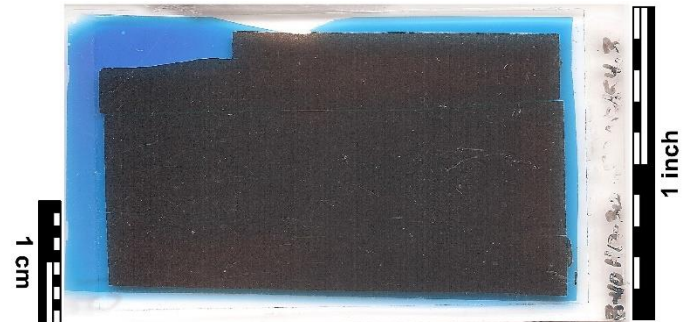
Thin section slide of dark gray pyritic carbon-rich shale Sample's high organic carbon content makes almost opaque. Blue epoxy impregnation indicates 0% porosity.
