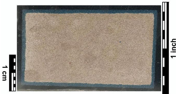
Billet of fine-grained quartz arenite sandstone Homogeneous, completely lacking lamination or other bedding features
