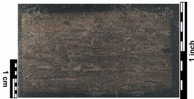
Billet of medium gray shale Sample rapidly absorbed water and puffed out of epoxy as splinters
