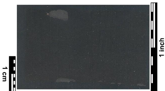
Billet of dark gray shale Homogeneous mudstone. Gray patches are air bubbles on sample surface.
