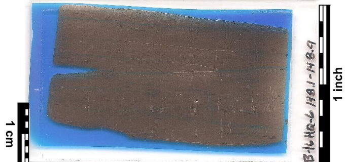
Thin section slide of medium gray pyritic shale Faintly bedded due to slight quartz silt variations. Blue epoxy impregnation indicates <0.1% porosity – mostly along shale partings.
