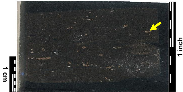
Billet of medium gray pyritic shale Note pyrite throughout sample (e.g., arrow)
