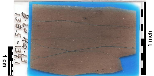
Thin section slide of gray shale Shale parts along irregular surfaces. 1 mm aggregate of very fine-grained pyrite near top center. Blue epoxy impregnation indicates 0% observable intergranular porosity, but detectable fracture porosity.
