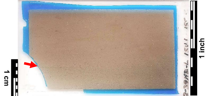
Thin section slide of light gray siltstone Slight grain size variation defines bedding (arrow) Blue epoxy impregnation indicates 0% porosity.
